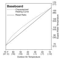
Not all heating terminal units behave in the same manner. Because of this fact, applying a generic outdoor reset strategy, such as a Reset Ratio, cannot provide the maximum performance and comfort from the heating system. A reset strategy that is customized to the heating system, such as a Characterized Heating Curve, will provide better performance and comfort.
