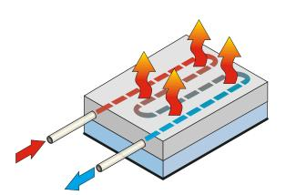
A radiant floor heating system is a closed loop system since the same fluid is heated, circulated and reheated through a piping loop, as opposed to open loop system to which fresh fluid with all of its associated gas and dissolved solids is constantly introduced. A domestic water application is an obvious example of an open loop system.
