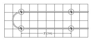
PEX tubing should be secured with tie straps every 3' (1m) on straight runs and at two points on a  $180^{\circ}$  bend.
