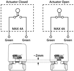
After ~2mm travel of the stem, the end switch is activated
