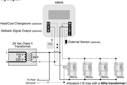
Note: If there are >5 actuators for 1 zone, it may be more cost effective to have a separate manifold and use an actuator on a zone valve.
