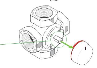
10. Attach the plastic adapter included in the 58131 package to the valve stem. The flat spot on the adapter will line up with the flat spot on the stem.
