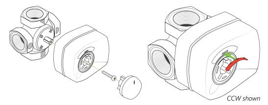
e. Ensure the knob is in the AUTO position. If not, turn the knob and push in until it "clicks" into place - no red should be visible around the base.
