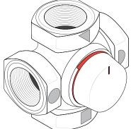
9. Remove and dispose of the factory mounted knob.
