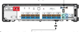
Step 3 Remove the rubber cap from the external antenna port on the bottom of the StatLink® 8 Zone Wireless Module.
