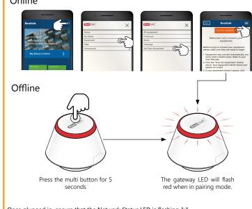
Once plugged in, ensure that the Network Status LED is flashing 1:1.
