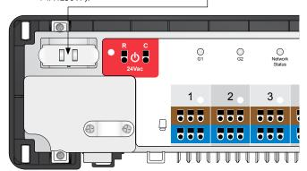
Step 7 Wire up to 3 actuators per zone, or 12 if using connectors; a total of 12 actuators can be wired to each module.
