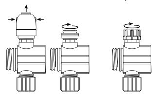
4. Insert the new shut-off shaft assembly.
